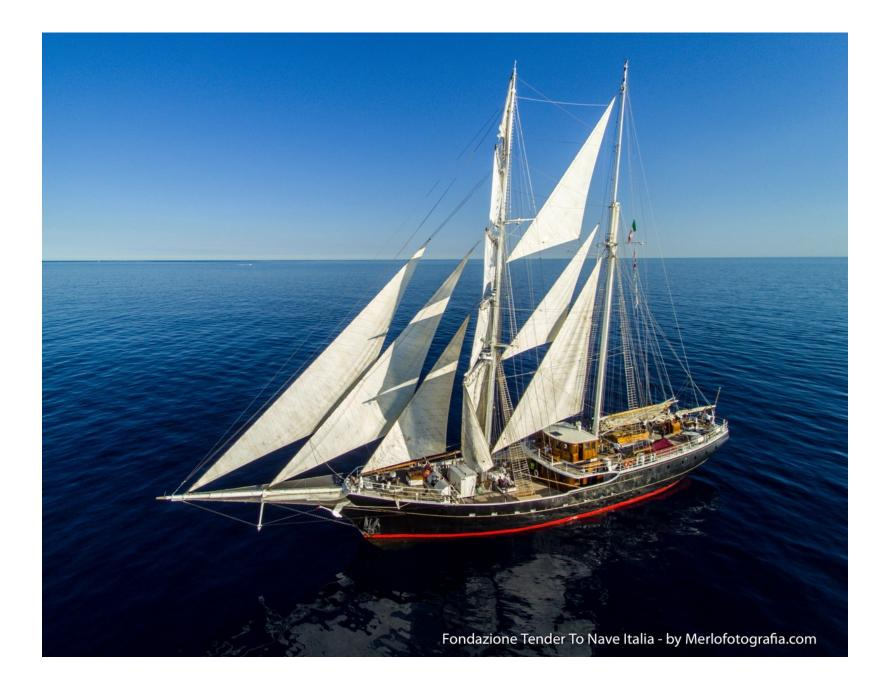
Lenght: 61 meters Width: 9,20 meters Draft: 3,80 meters Displacement: 480 tons Crew: 21 military
